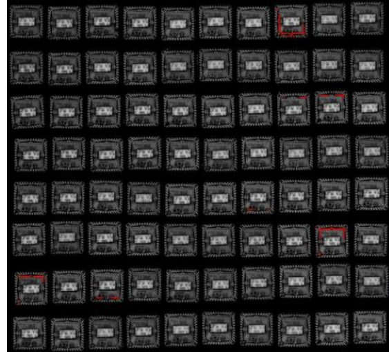
Unit Position no. 1 – 80 C-SAM Top (Reflected Mode) Results : No Delamination
