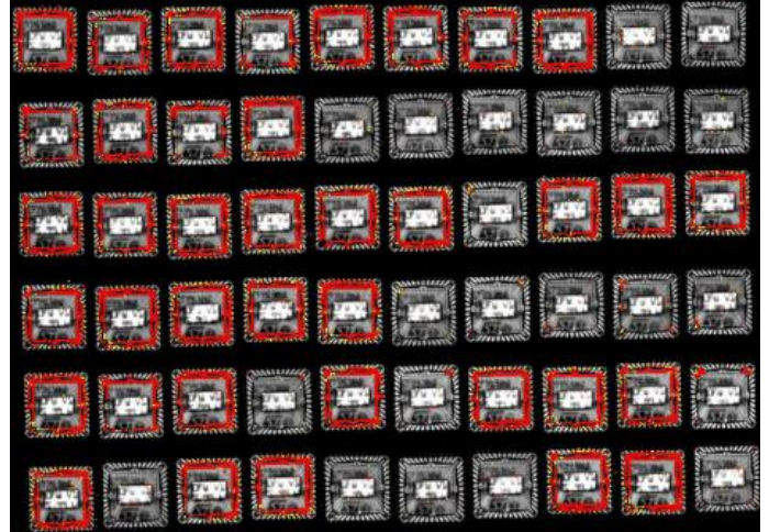
Unit Position no. 1 – 60 C-SAM Top (Reflected Mode) Results : No Delamination
