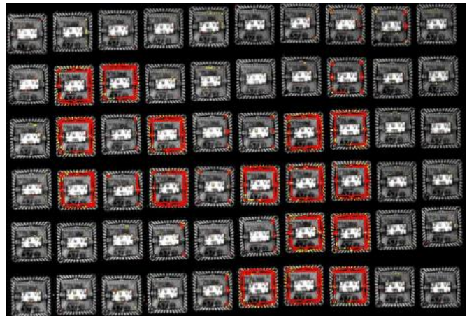
Unit Position no. 1 – 60 C-SAM Top (Reflected Mode) Results : No Delamination
